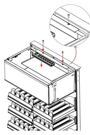
Secure Cord Management Tray with (2x) #10-24 X 3/4" bolts. The plug strip can then be placed on top of the tray.
