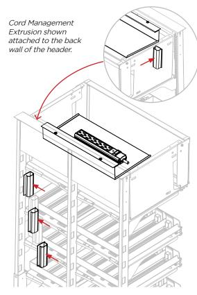
3. Peel protective backer off tape to apply Cord Management Extrusions where needed. They can be applied along the back inside areas of the uprights and to the back wall of the header areas, as shown above.
