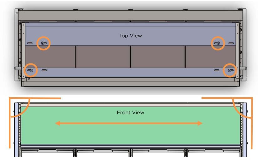
To square up end panels, loosen the bolts and wing nuts attaching the header to fixture shelves. Slide header to left or right square up and tighten wing nuts and bolts to secure header in place.
