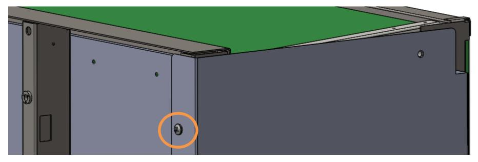
Align hole on back of end panel with weld stud on back of fixture upright. Attach with provided hardware (details on next page).
