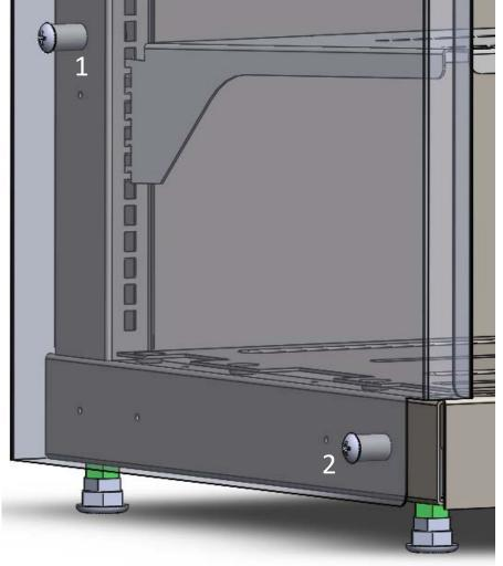
Attach the bottom of the end panel using long through bolts (2-1/2"), short spacers (11/16"), and keps nut in the two locations shown. Spacer install between the end panel and fixture leg.
