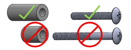
Align hole in top corner of end panel with matching hole in header assembly. Attach using shorter through bolt (1-3/4"), long spacer (1-1/4"), and keps nut.
