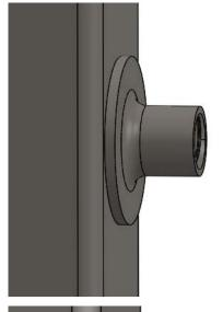
Identify weld stud style on back of fixture upright.
