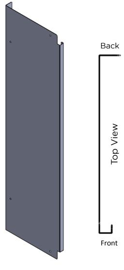
Upper and lower panels can be installed on either side of a fixture. They are "non-handed" parts. Simply flip the panel for use on the opposite side.
