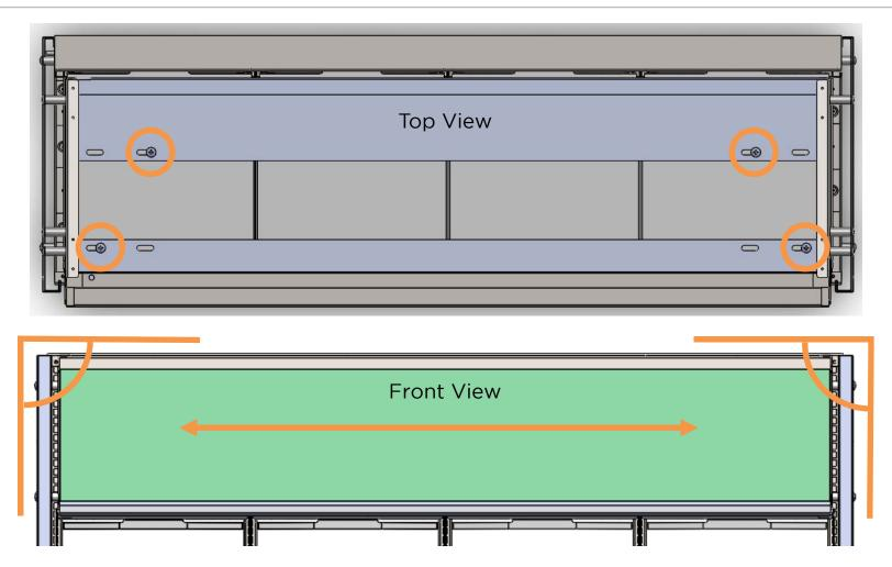
To square up end panels, loosen the bolts and wing nuts attaching the header to fixture shelves. Slide header to left or right square up and tighten wing nuts and bolts to secure header in place.
