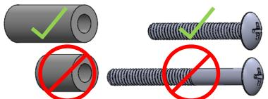
Align holes in Upper Panel with slotted holes in Header. Hang upper panel using shorter through bolts (1 ¾"), long spacers (1 ¼"), and keps nuts.
