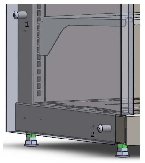
Hang lower panel using long through bolts (2 ½"), short spacers (11/16"), and keps nuts in the two location shown. Spacers install between End Panel and fixture leg.
