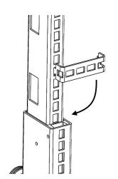
2. Rotate & push bottom 3. Push down flush into hole above lower leg
