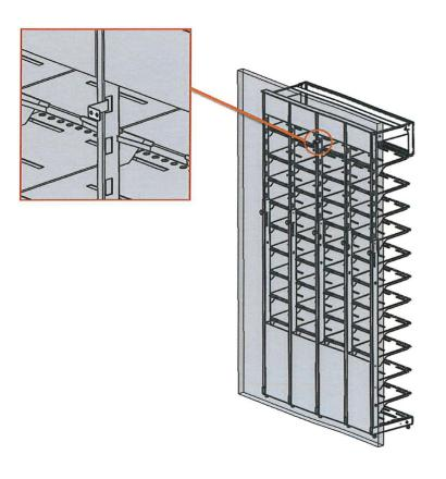
Alternative mounting method: Using cable, wall mount, screws and anchors.
