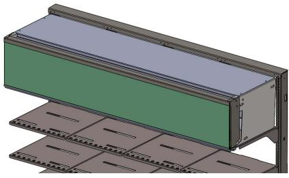
Position Top Cap with bent edge facing towards front of fixture as shown. Align holes on each side with holes in top of header box and secure with provided hardware.
