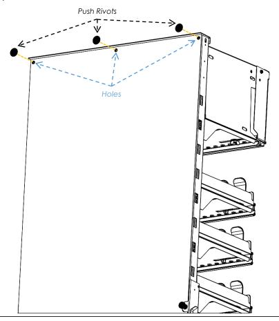
**NOTE**: If Back Panel is longer than the height of the display, it needs to be trimmed. Please trim off the bottom edge by scoring it with a knife and then snapping off excess material.
