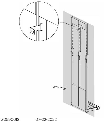
Alternative mounting method: using wire cable, wall mount, screws and anchors.
