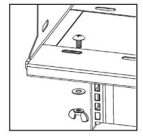
NOTE: Headers can be installed in any location on fixture, even across fixture connection points.
