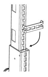
2. Rotate & push bottom into hole above lower leg.
