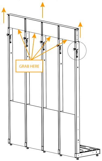
3. Tighten Lock Knobs. When the fixture is at the desired height, the lock knobs MUST be tightened.
