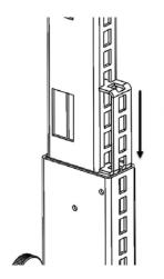
Slot Extension Bracket allows for a shelf to be placed at the point where the Infinity Fixture telescopes.
